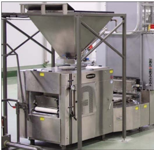
Above: Adamatic VDR Divider Rounder with Bulk Hopper / Bowl Lift as part of Adamatic Roll Makeup Line
